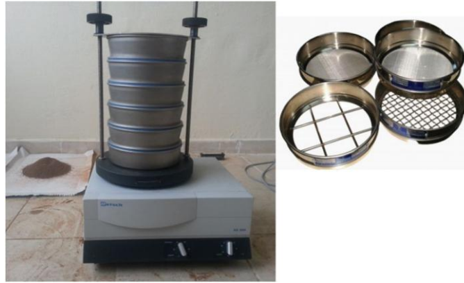
Figure 3. Sieve shaking device and sieve set
