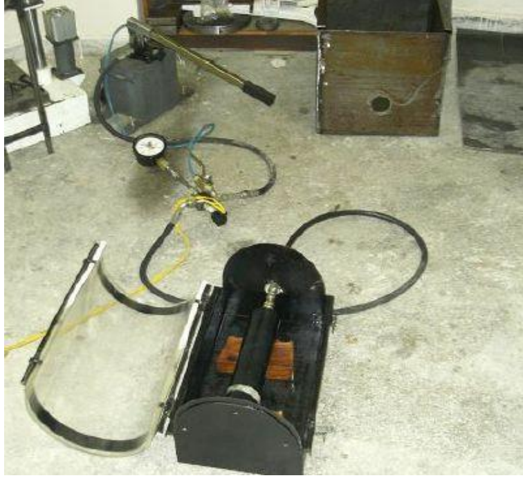
Figure 4. Free-end static internal pressure burst test unit (Demirci, 2015).
